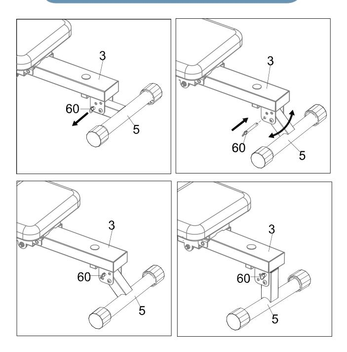
**3A.** Adjust the angle of **Rear Stabilizer (5).** There are three holes for different angle options.
