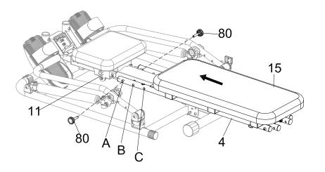
Loosen the Knobs (80), and adjust the Backrest (15) to the suitable position A, B or C. Lock the Knobs (80).
