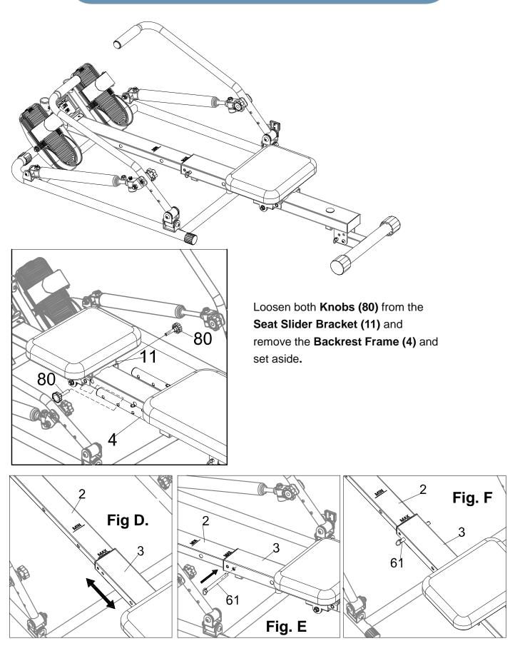
2A. Adjust the Slide Tube (3) to a comfortable position for your height at MIN or MAX. See Fig. D.
