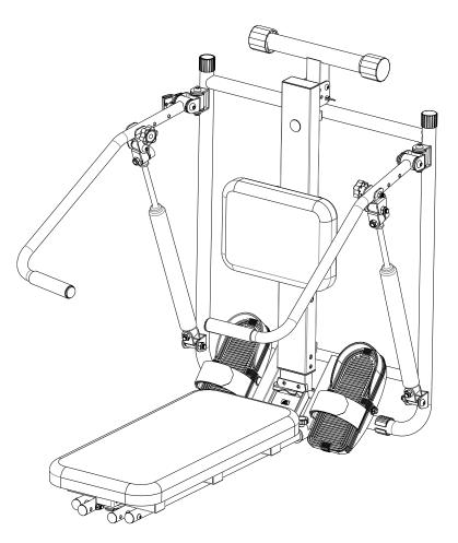
**5A.** Lay the Rower down on the **Backrest (15)** and adjust the **Seat (16)** onto the upper position then insert the **Pin (61)** to secure it.
