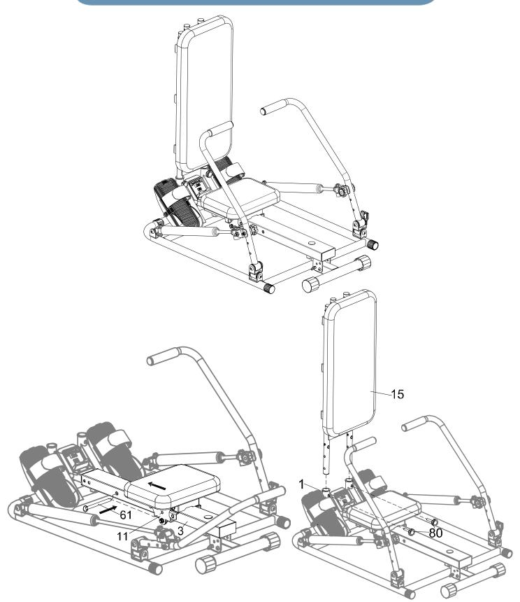
**4A.** Move the **Seat Slider Bracket (11)** to the pedal position, align the hole and insert the **Pin (61)** to secure it.
