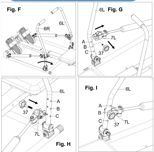
You may adjust the **RESISTANCE** to a suitable position. **A**. is the highest resistance setting. **B**. is middle resistance setting. **C**. is the lowest resistance setting.
