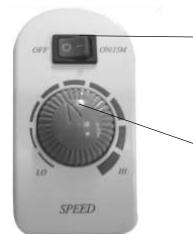
ACTIV cycle is on a 15-minute timer after turned on. Turn power switch OFF and ON again to restart 15-minute timer.
