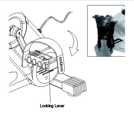
Pull Locking Lever fully to unlock pedal to unfold the pedals.
