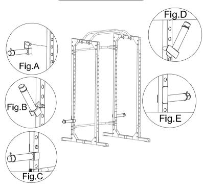
Bring the Weight Horn to the area near Rear Cross Bar (K). See Fig A. Slide it into the holes of the Upright Frame (B) at a 90-degree angle. See Fig B. Release the attachment and it will be in place. See Fig C.
