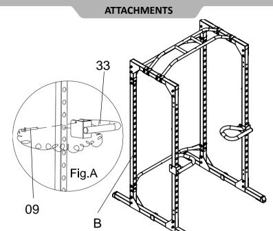
Bring the Dip Bar (33) to desired height. Slide the attachment into the holes of the Upright Frame (B) at desired height. Then secure the attachment by inserting Pin I (09).
