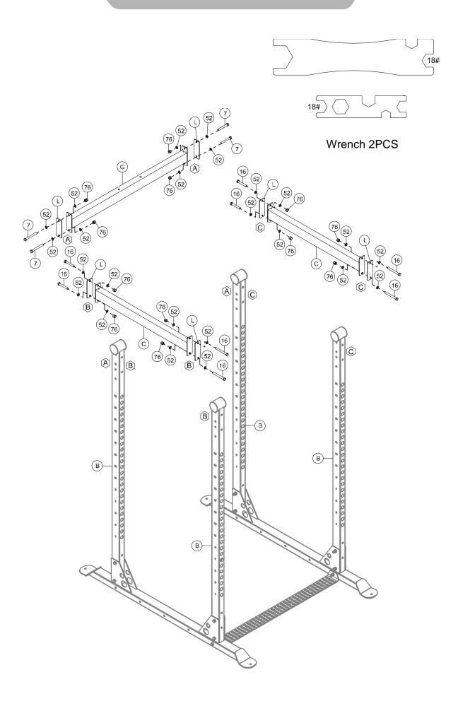
4A. Attach the **Front Crossbeam (D)** and the two **Mounting Plates (L)** to the two front **Vertical Posts (B)** at the location of the matching D by using:
