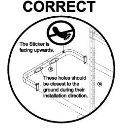
Now that the cage is fully assembled, proceed with thoroughly tightening all the hardware.
