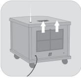
2. Gently remove the air filter from the rear of the heater.
