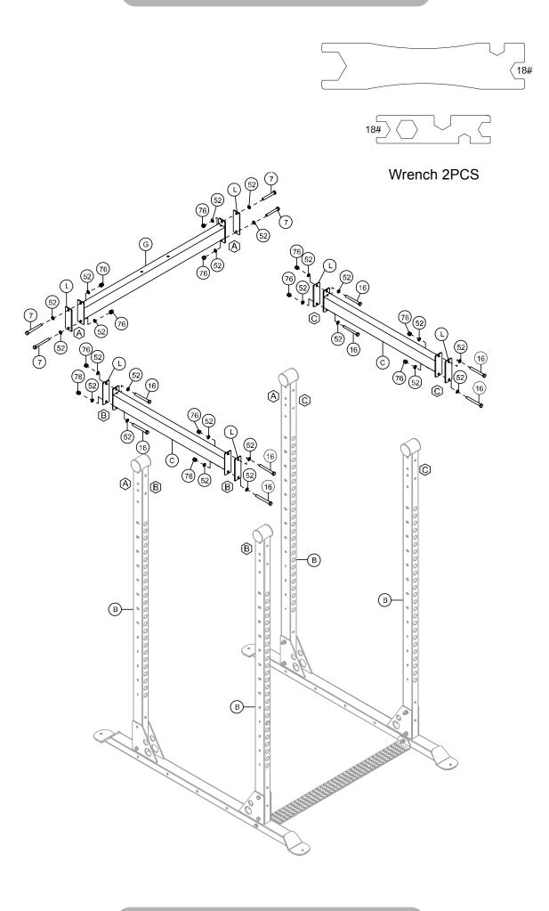
4A. Attach the Front Crossbeam (D) and the two Mounting Plates (L) to the two front Vertical Posts (B) at the location of the matching (D) by using:
