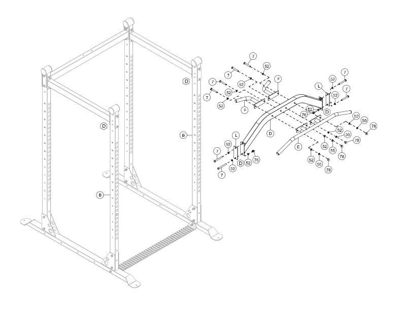
5A. Attach the Stability Beam (K) and the two Mounting Plates (L) to the two rear Vertical Posts (B) by using:
